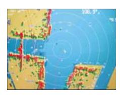
Radar overlav Radar targets can be overlaid onto the electronic chart so that you can better recognize what's around your vessel by referencing the target locations on both the chart and the radar.
